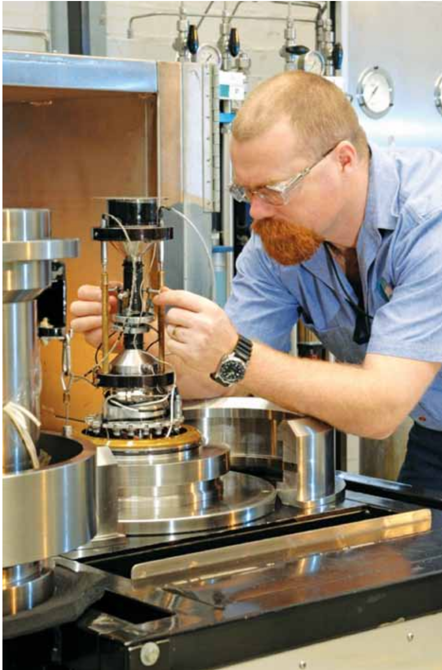
Testing core samples at the CSIRO laboratory in Bentley. Photo courtesy CSIRO
