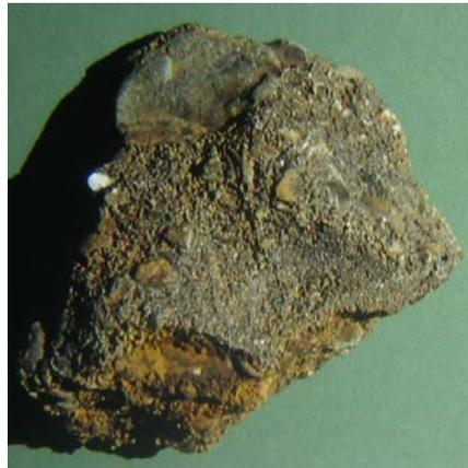
Figure 3.20: Holocene sediment of the Rhine river, cemented by iron oxy-hydrate near the mineral springs of Rhens.
