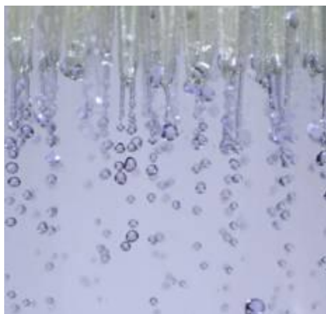
Figure 8. Droplets forming in basic solution pumped through pipette tips attached to the upper flange and falling into the glass gas reactor. High resolution images were used to determine average droplet shape and size.
