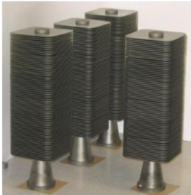
Figure 6 – Planar wafer ITM ceramic membrane stacks from Air Products & Chemicals (USA).
