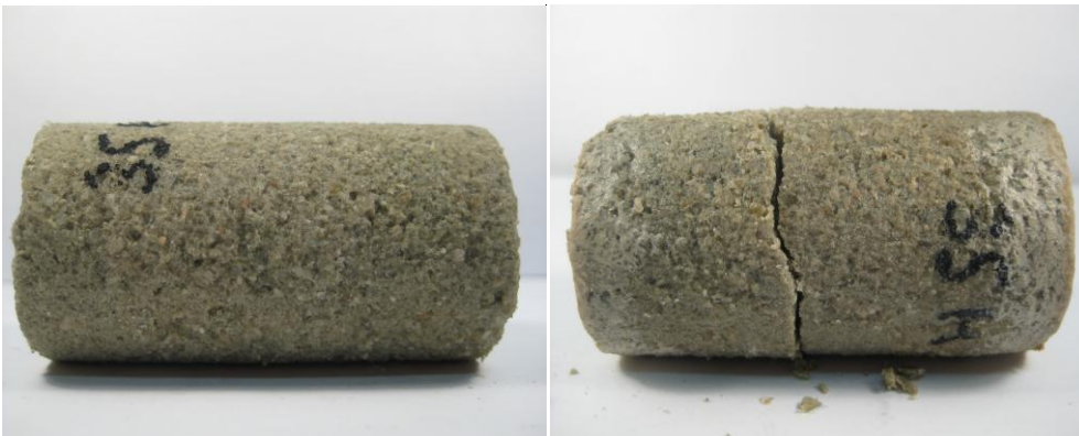
Sample 206635 (1323.93) before (left) and after (right) geomechanical testing
