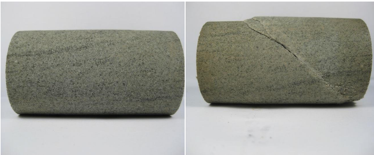
Sample 206662 (1940.58) before (left) and after (right) geomechanical testing
