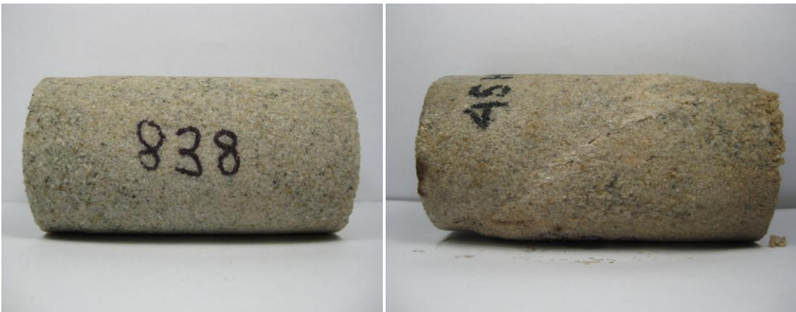
Sample 206645 (1897.66) before (left) and after (right) geomechanical testing
