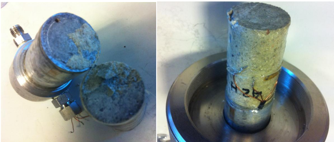
Figure 7.11. Top and bottom of sample 206642 broken in the Hoek's cell under a confining pressure of \sim 10 MPa.
