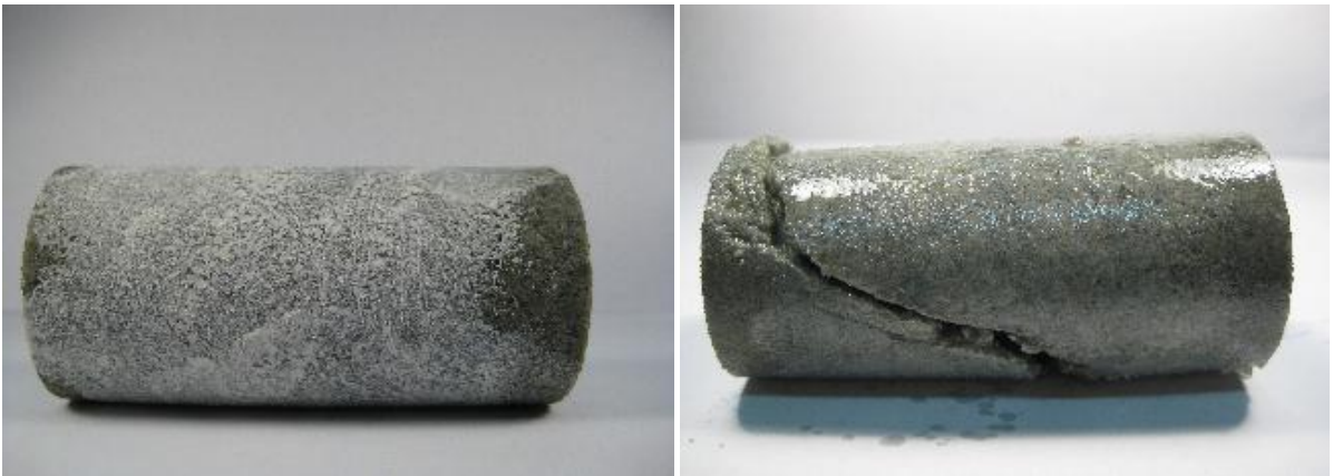
Sample 206683 (2516.00) before (left) and after (right) geomechanical testing
