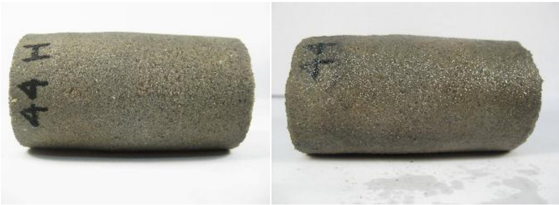
Sample 206644 (1343.61) before (left) and after (right) geomechanical testing
