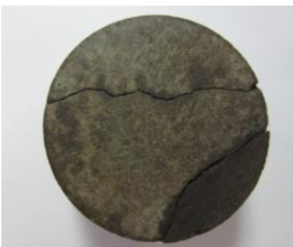
Figure 5.5 Cross-sectional view of the shale disk showing the fractures induced during sample preparation (sample diameter=3.8 cm)
