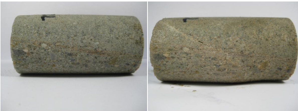
Sample 206672 (2496.22) before (left) and after (right) geomechanical testing
