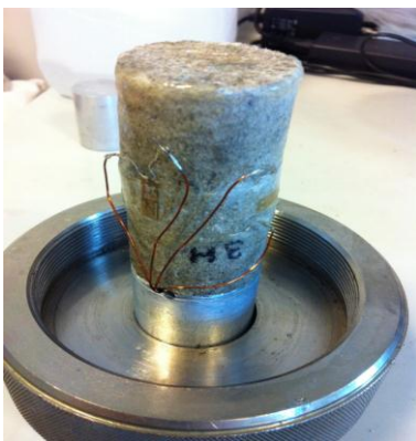
Figure 7.2. Sandstone sample 206603 with radial and axial strain gauges glued to its surface.
