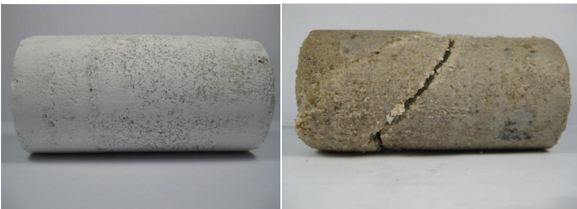
Sample 206646 (1897.91) before (left) and after (right) geomechanical testing
