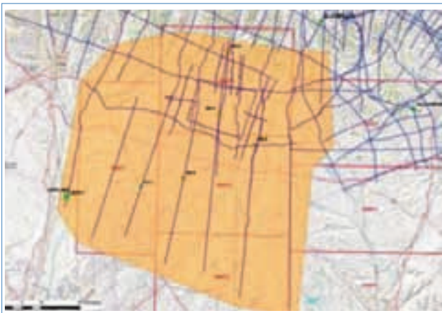
Figure 4.10 Static model (orange polygon). Seismic surveys are plotted in purple, old wells in green, new wells in yellow (deep wells) or blue (shallow wells); red polygons are ENDESA permit boundaries
