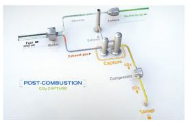
a high purity  ${\rm CO_2}$  stream. This technology is widely used to capture  ${\rm CO_2}$  for use in the food and beverage industry.
