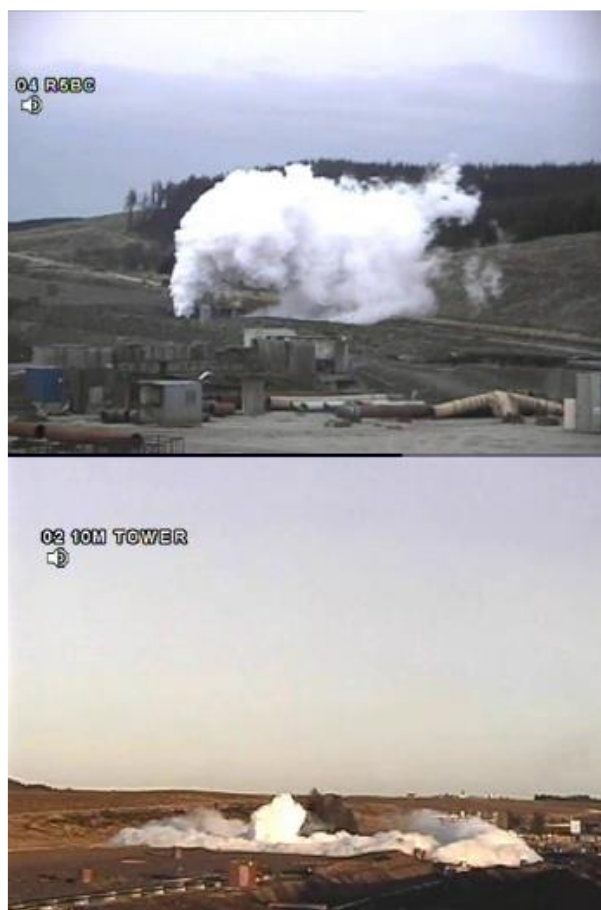
Figure 8.3: Vertical discharge versus 'blanket' formation
