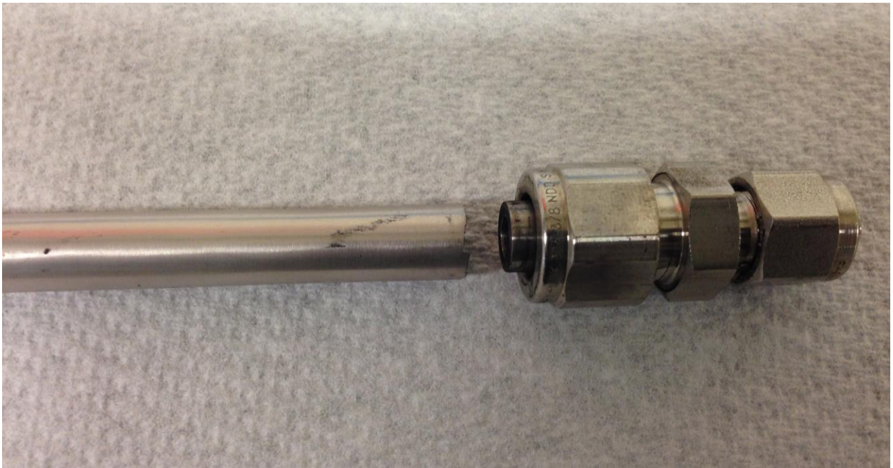
Figure 10: Fractured membrane after CMR test due to physical restriction caused by the catalyst bed against membrane expansion
