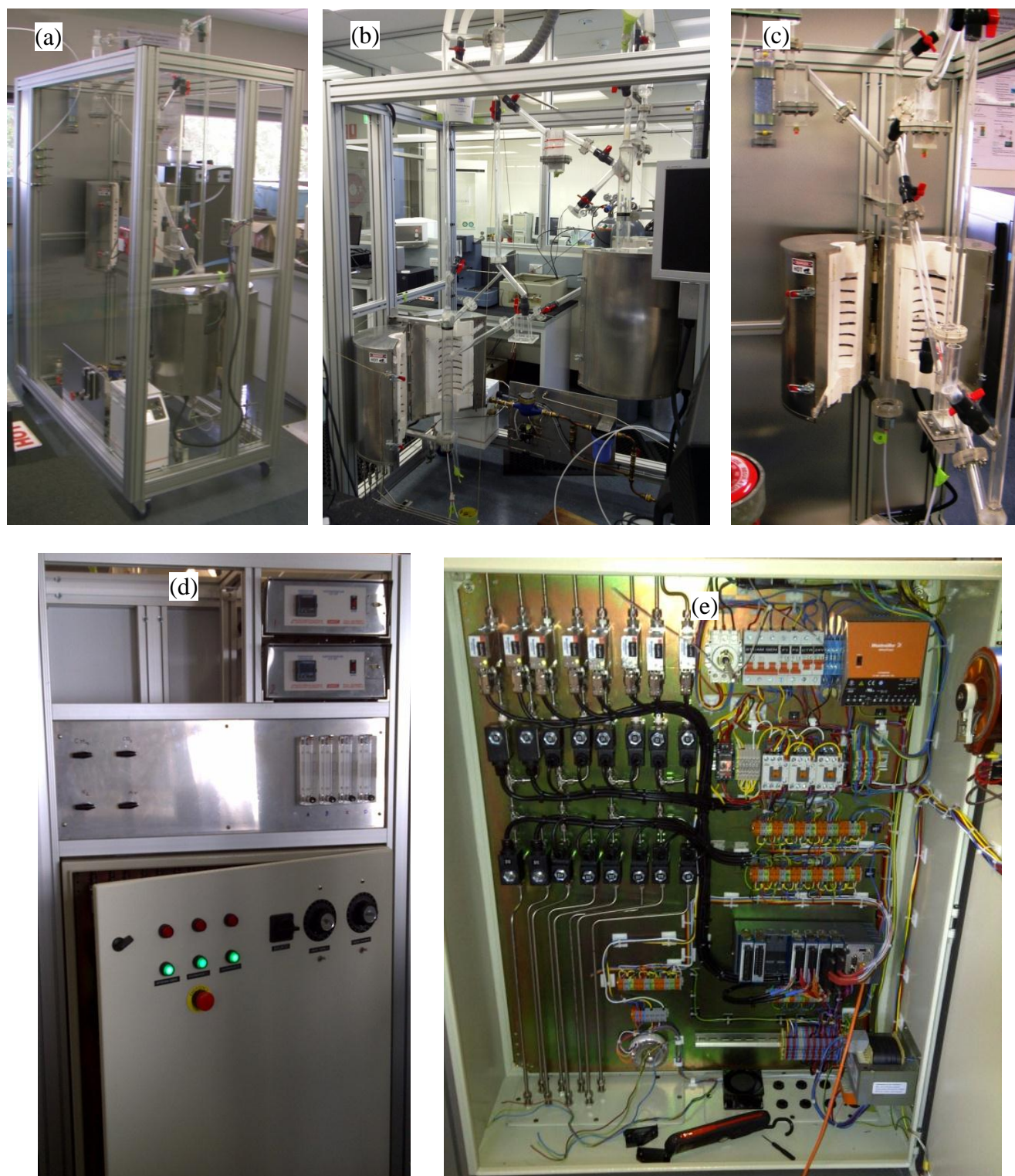
Figure 7: Pilot plant; (a) full assembly, (b) full assembly front view, (c) enlarged view of a Perspex vessel and tube furnace, (d) control box, (e) internal view of the control box.
