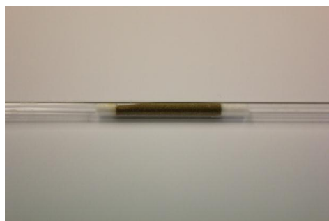
Figure 10: Photograph of the quartz tube reactor loaded with a metal oxide sample.
