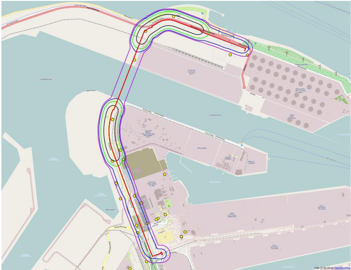
Figure 3.6: Individual risk contours: failure of high pressure CO 2 pipeline with worst case risk of consequential failure of the nearby gas pipeline
