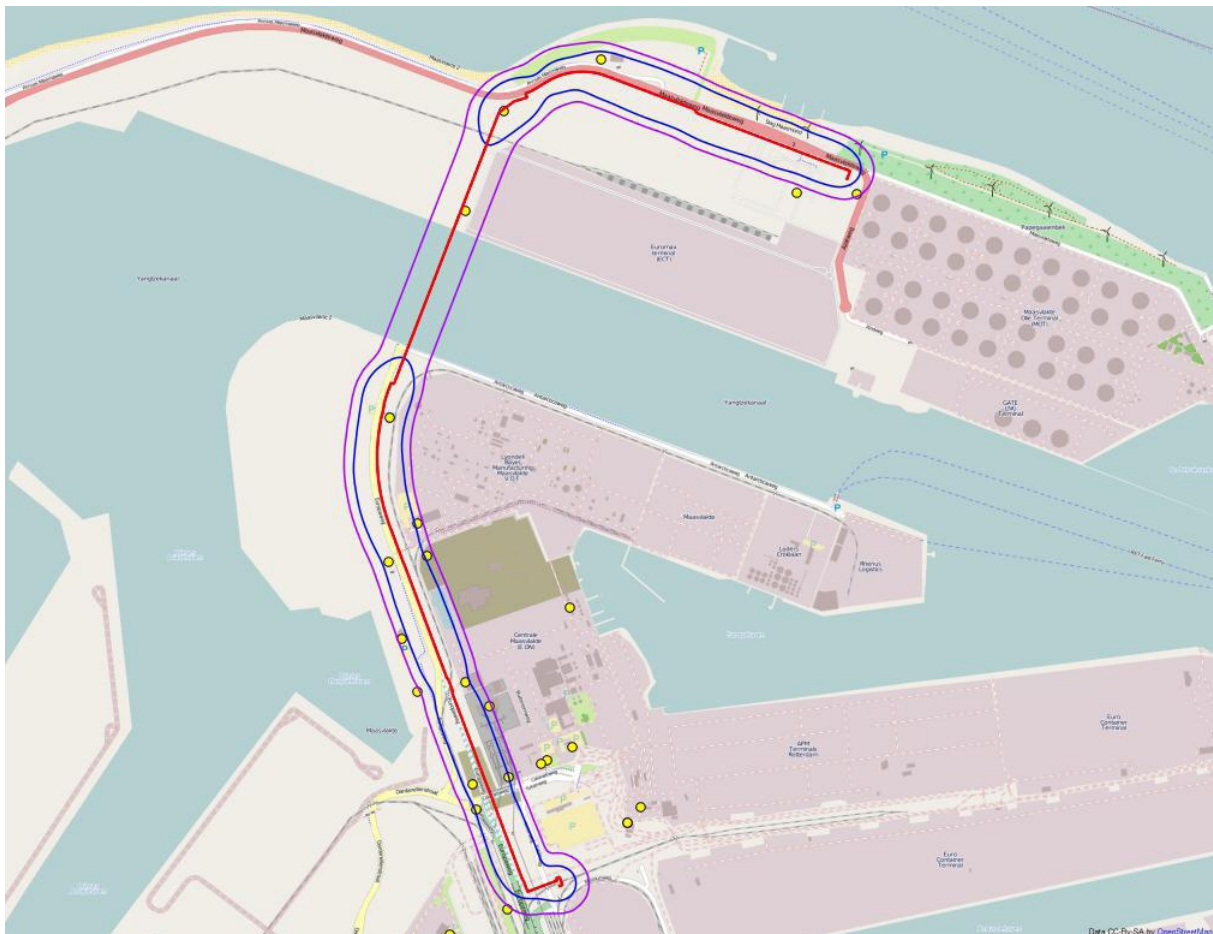
Figure 3.5: Individual risk contours (failure of high pressure CO 2 pipeline without nearby pipelines)
