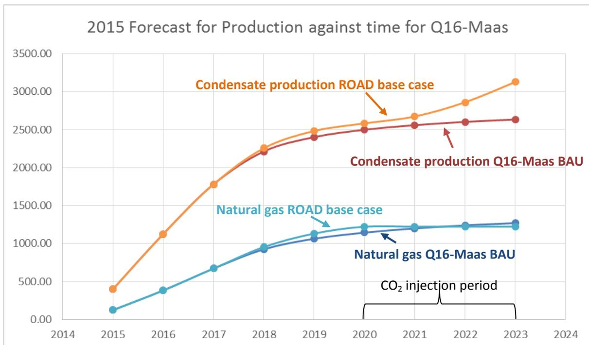
Figure 11.1 2015 Cumulative production forecast for Q16-Maas (mln Nm<sup>3</sup> gas and k stb condensate)
