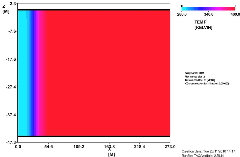
To understand the effect of the temperature of the injected CO<sub>2</sub> on the reservoir two injection scenarios were studied, a “warm” injection scenario with a bottom hole temperature (BHT) of 285 K and a “cold” scenario with a BHT of 259 K.
