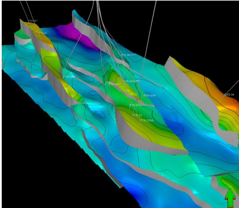
The P18-4 gas reservoir is suitable geological structure for CO<sub>2</sub> storage because:
