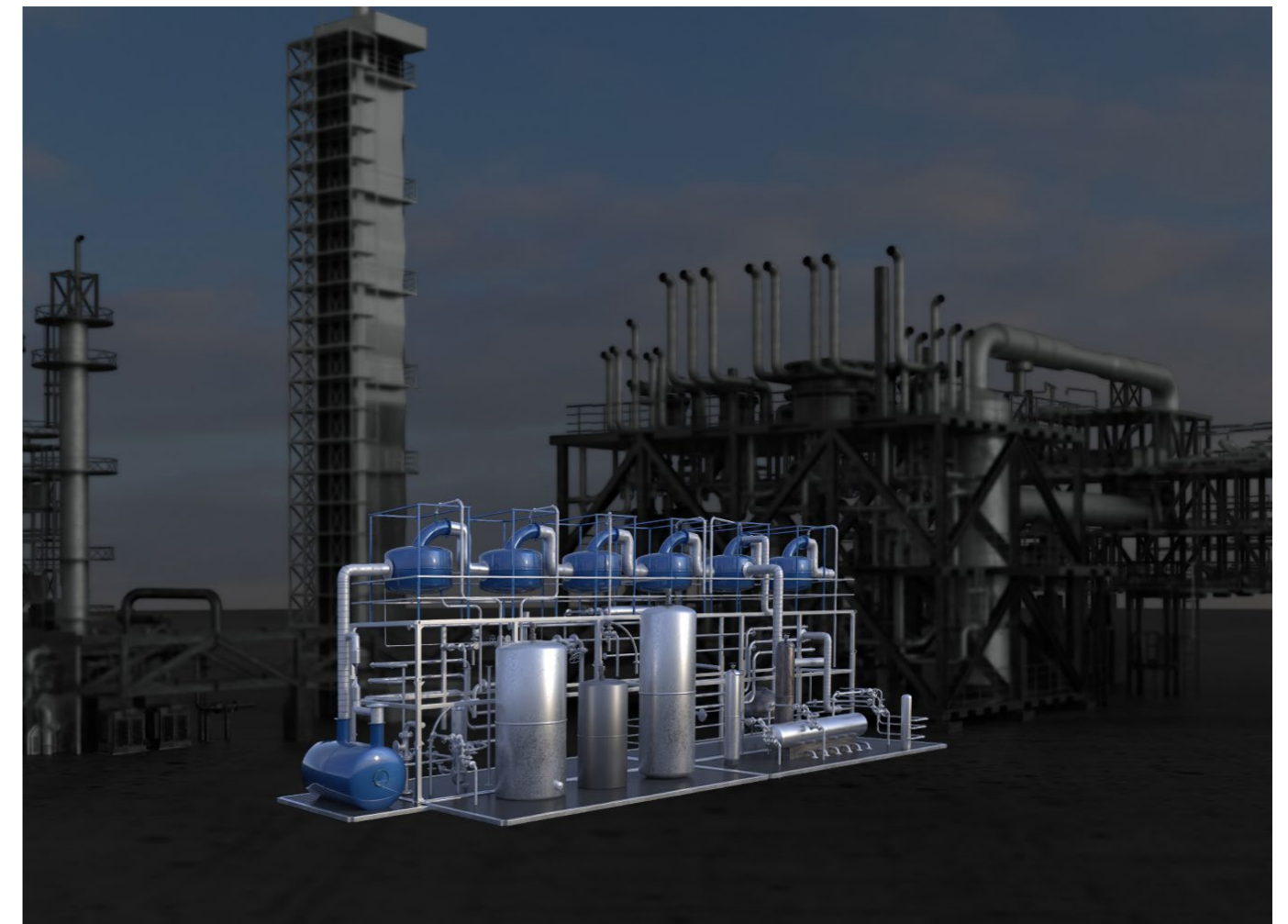
CycloneCC 100 TPD visualisation showing its relative size compared to a conventional carbon capture plant
