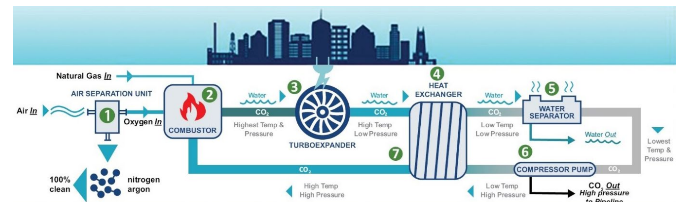
Figure 1: The NET Power Process
