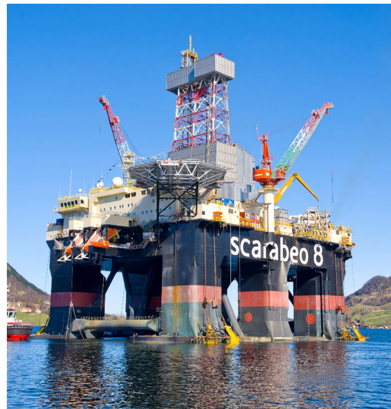
Saipem Scarabeo 8, a last generation semisubmersible drilling rig
