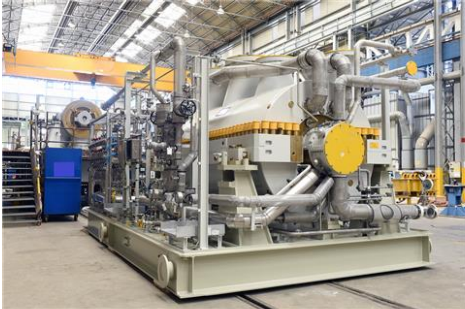
CO 2 compressor for Santos' Moomba CCS Project Source: Baker Hughes
