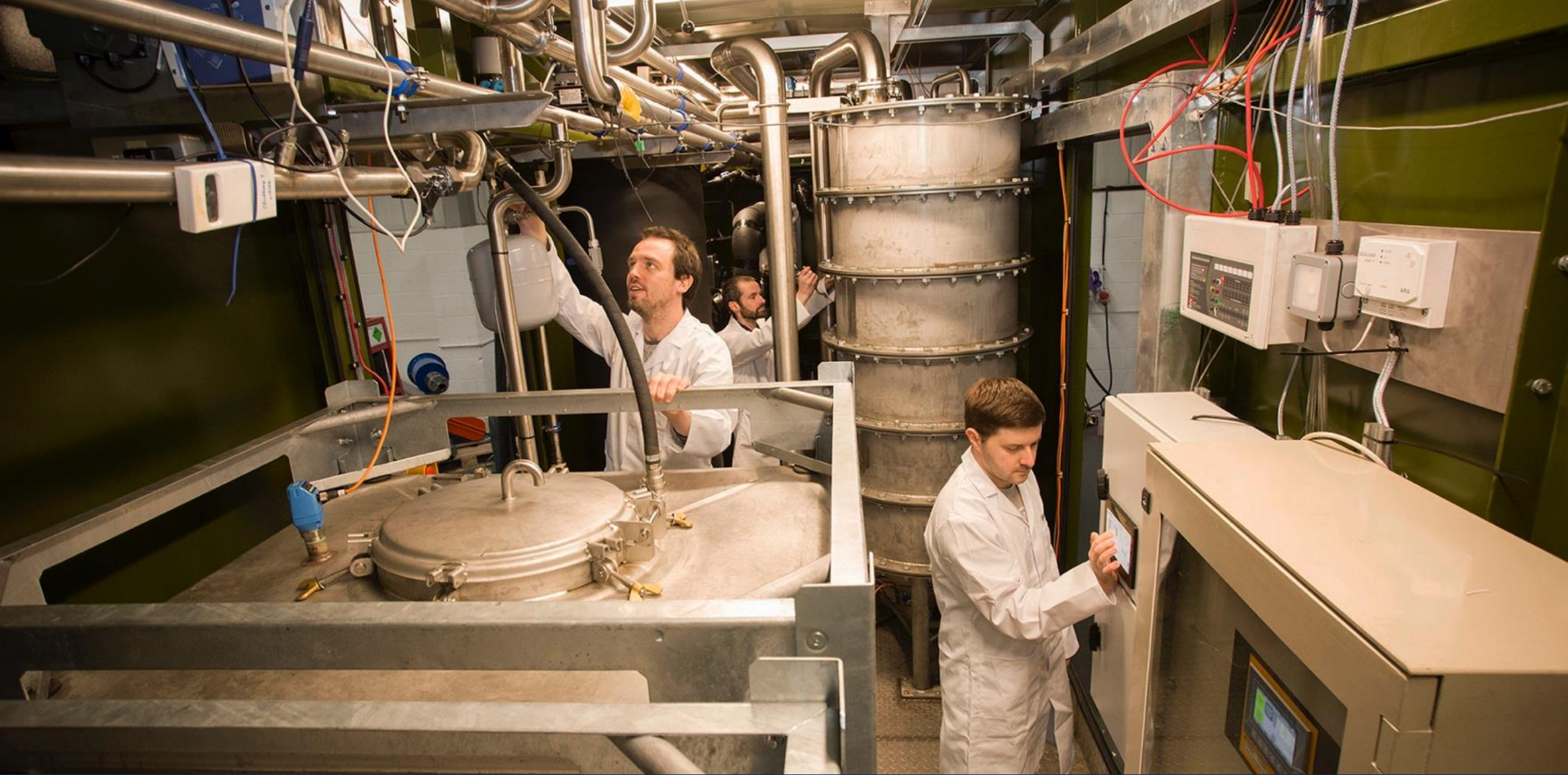
This shows the inside of the shipping container during the biogas trials. In these trials we used a bubble absorber which can be seen in the background
