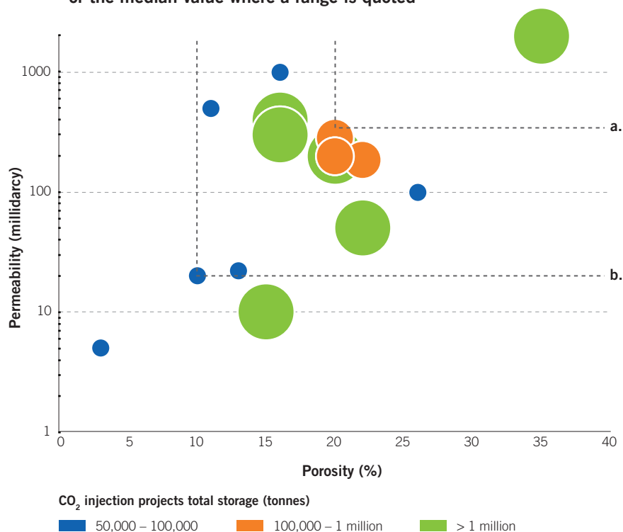
Figure 3.7 Reservoir porosity and permeability of storage projects. Trend lines are the minimum limits for site selection criteria according to a. Chadwick et al. 28 b. IEAGHG 29 . Note: The average porosity and permeability value has been used where reported, or the median value where a range is quoted
