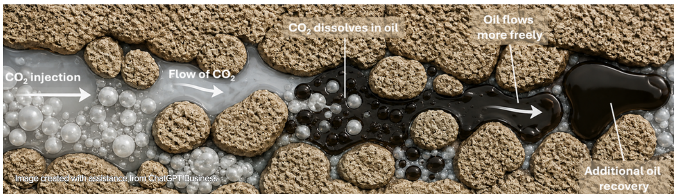
Figure 2. Microscopic conceptualisation of CO 2 moving through rock pore spaces, dissolving into the oil, and reducing its viscosity to enable recovery
